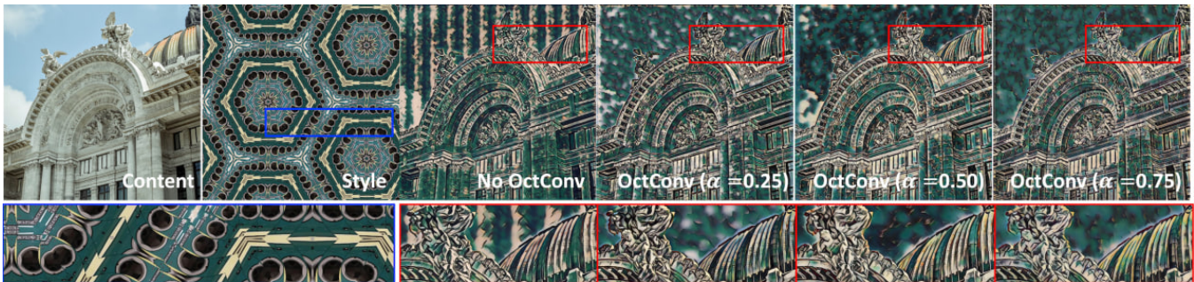
Figure 2: The stylization outputs with no octave convolutions and octave convolutions in different alpha values. Alpha values ( \alpha ) denotes the ratio of the number of low-frequency channels to the total-frequency channels.
